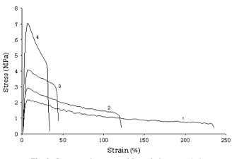
Fig. 3. Stress-strain curves of formulations nos. 1-4
