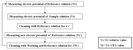
Fig. 1. Measuring process by the electronic tongue
